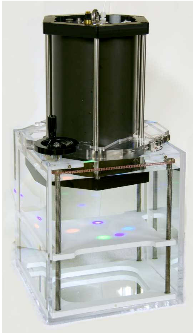
Fixture with HydroScat-6P, ready for calibration (plaque not shown).
